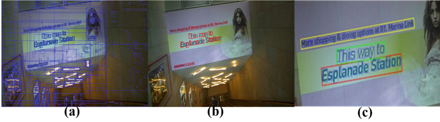
Fig. 4. The result of text line formation: (a) text candidates detection result, (b) text components after removing non-text components, (c) text line detection result.
