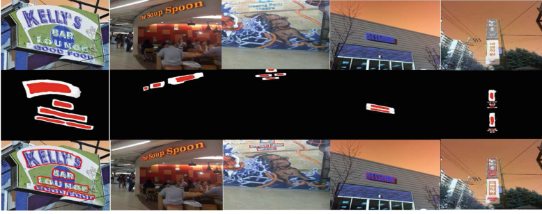
Fig. 1. Scene text detection results achieved by the proposed TK-Text. For text of arbitrary orientations and shapes in first row , TK-Text first predicts text kernel segmentation (in red color) and rough text segmentation (in white color) as shown in second row , and then draws bounding box for text instances as shown in third row . (Color figure online)
