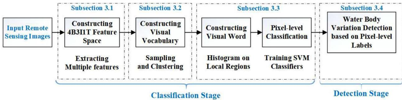
**Fig. 1** Workflow of the proposed water body variation detection algorithm, which consists of two stages, i.e., classification and detection
