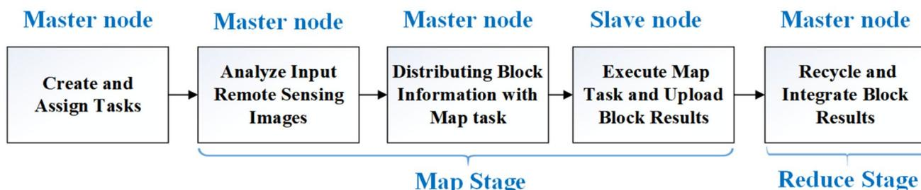
**Fig. 4** Workflow of water body variation detection method with distributed processing, which utilizes MapReduce structure to facilitate parallel running
