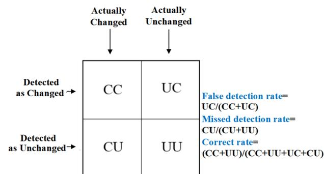
**Fig. 6** Explanation on the adopted measurements to evaluate performance of water body variation detection
