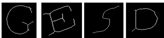
Fig. 10 Filtering false medial axis segments
